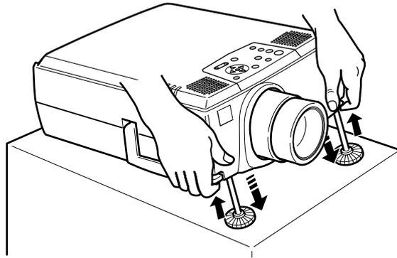
2. While lifting the levers, raise or lower the projector until the screen image is correctly positioned.
