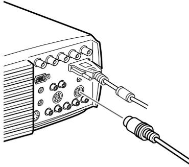
2. To use the remote control as a wireless mouse, connect the PS/2 or USB cable included with the projector to the MOUSE terminal on the square end of the main cable.
