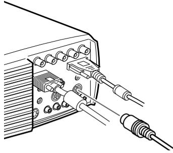
2. To use the remote control as a wireless mouse, connect the PS/2 mouse or USB cable included with the projector to the MOUSE terminal on the square end of the main cable.
