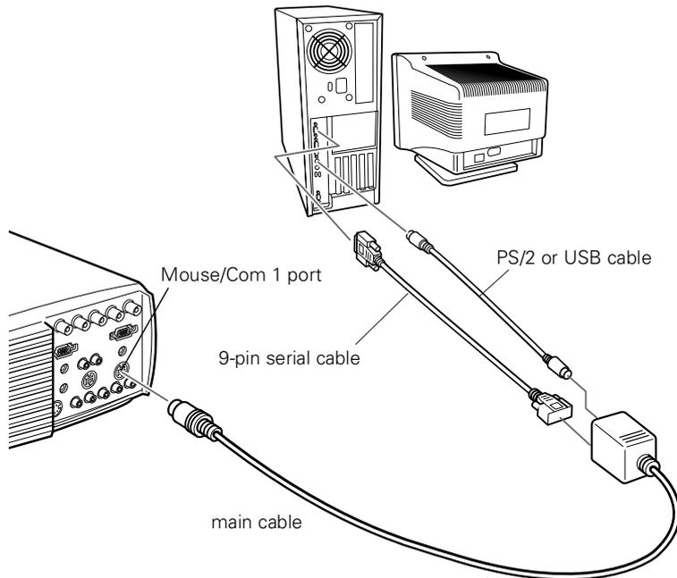
1. Connect the round end of the main cable to the projector's Mouse/Com 1 port. (Use the Mouse/Com 2 port if you are connecting a second computer.)
