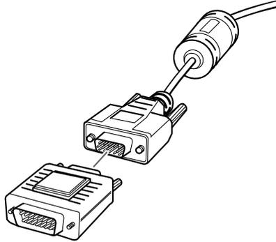
4. Disconnect the monitor cable from the video port on the back of the Macintosh. Then connect the projector video cable (with the Macintosh desktop adapter attached) to the video port on the Macintosh.
