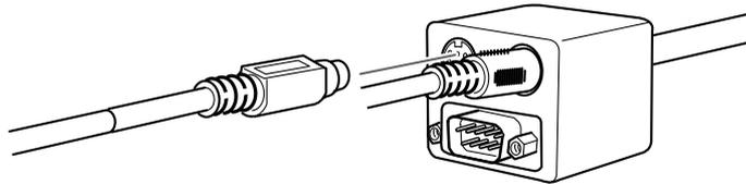
5. Connect the other end of the serial cable to the
