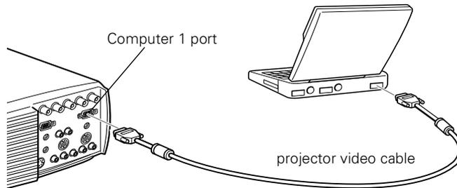
1. Connect one end of the projector video cable to the projector's Computer 1 port. (Use the Computer 2 port if you are connecting a second computer.)
