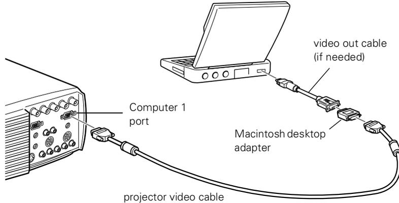
*Note: Some new PowerBooks may allow you to connect the video cable directly to the computer without using a video-out cable. See your PowerBook manual for additional information on connecting a video cable.*
