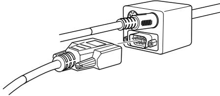
Connect the other end of the serial cable to the serial port on the back of your computer.
