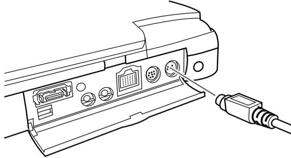
4. To use the ELP Link IV software or program new effects for the Effects buttons on the remote control, connect one end of the Mac serial cable to the MAC SERIAL terminal on the large end of the main cable.
