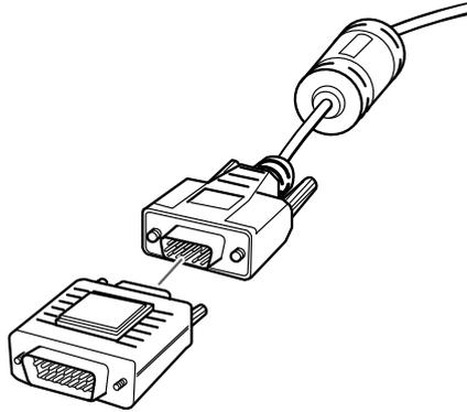
4. Connect the projector video cable (with the Macintosh desktop adapter attached) to the video-out port on the PowerBook.
