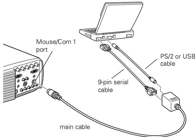
1. Connect the round end of the main cable to the projector's Mouse/Com 1 port. (Use the Mouse/Com 2 port if you are connecting a second computer.)
