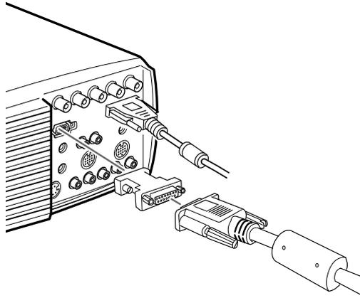
6. Tighten the screws on all the connectors.
