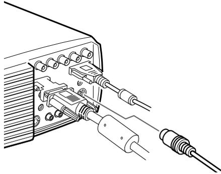
2. To use the remote control as a wireless mouse, connect one end of the projector's Mac mouse or USB cable to the MOUSE terminal on the large end of the main cable.
