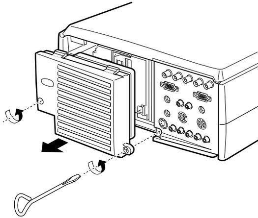
4. Use a screwdriver to loosen the three screws holding the lamp unit in place. (You cannot remove these screws.)
