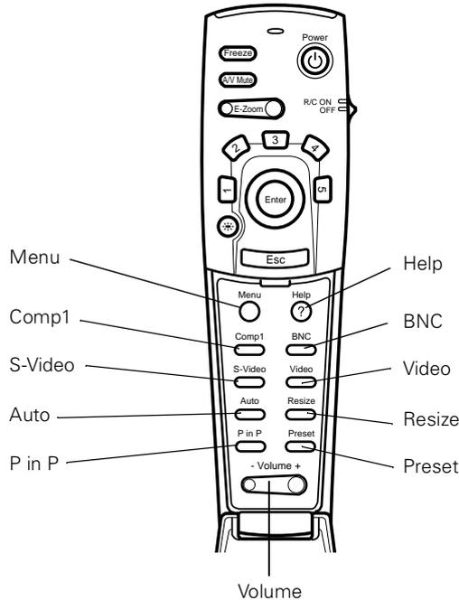
The remote control uses a line-of-sight infrared signal. To use the remote control, point it toward one of the remote control receivers located at the front and back of the projector. (See page 62.)
