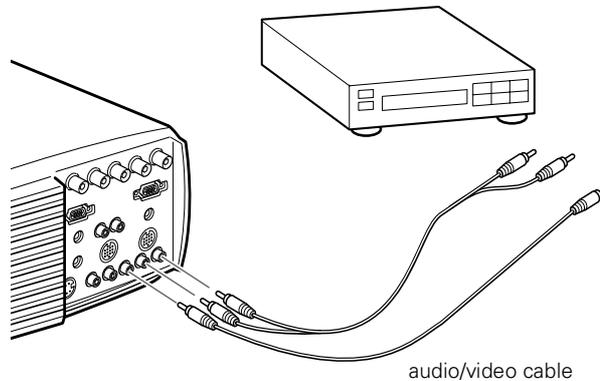
4. Connect the RCA audio cable to the Audio ports of the projector: insert the white plug into the L port and the red plug into the R port. Connect the plug at the other end of the RCA audio cable to the audio output ports of the video source.
