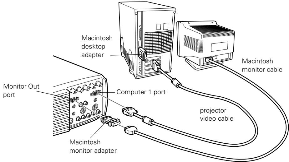
1. Connect one end of the projector video cable to the projector's Computer 1 port. (Use the Computer 2 port if you are connecting a second computer.)
