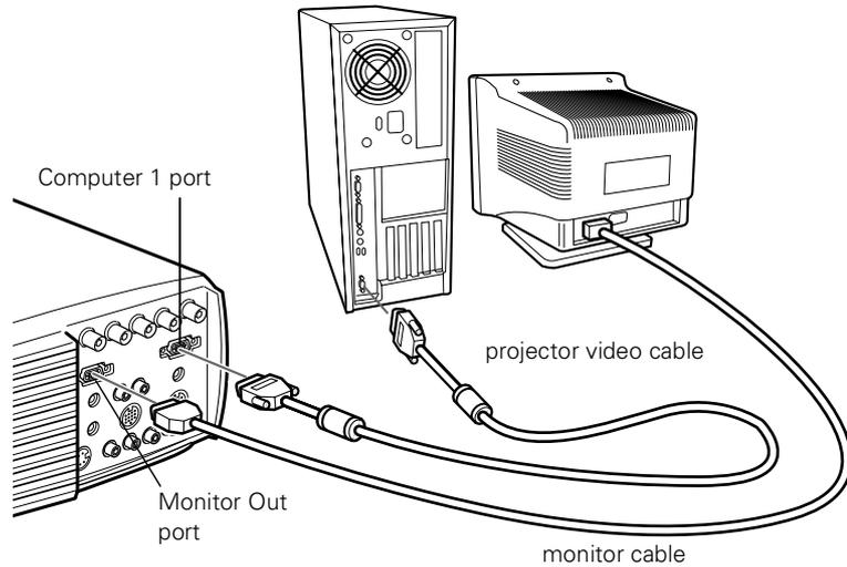
1. If you will be viewing the video on your computer monitor as well as the projector screen, disconnect the monitor cable from the video port on the back of your computer. Then connect the monitor cable to the projector's MONITOR Out port, as shown below. (This is useful when you need to view the video output but the projection screen is behind you.)
