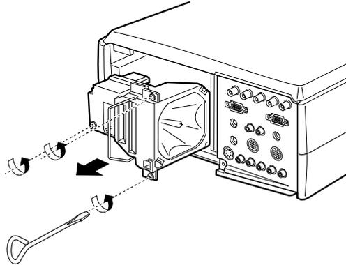
5. Lift up the handle and pull out the lamp unit.
